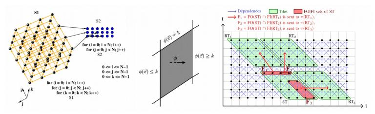
PLUTO is an automatic parallelization tool based on the Polyhedral Model to optimize arbitrarily nested loop sequences with affine dependencies
